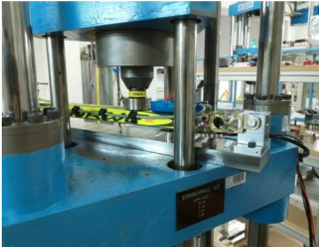
Figure 7.2 Roller ski test measurements in progress at a 20 kN force standard at VTT MIKES in Kajaani.
